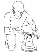
Figure 41-E. Slump Test (Cone Invert)
